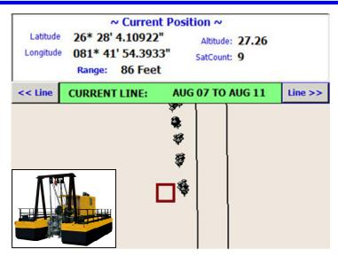
The LAS Dredge Monitor is ideally suited for use in dredges to increase productivity, and in any water based vehicle which is required to follow a designated course. If production lines - such as the dated line pictured above - are entered into the system, the vehicle's distance from the currently selected line is automatically calculated and displayed on the screen.
